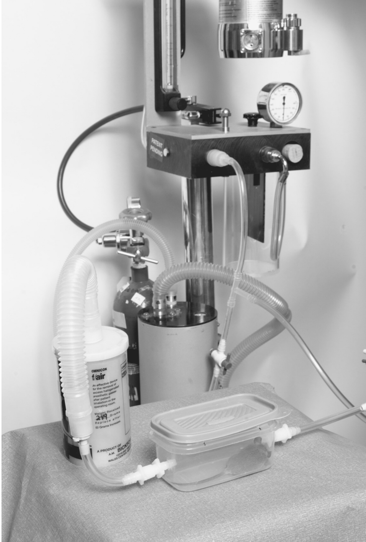
Fig. 4.15 A typical setup for inhalation anesthesia of mice with a commercially available precision vaporizer with homemade induction chamber for induction of anesthesia.
